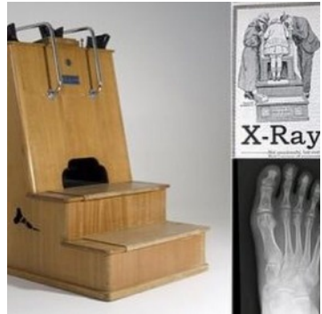
Fluoroscope shoe-fitting machine (image from the web)
