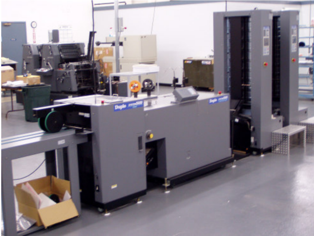
This machine collates, folds, stitches, and trims the NA
